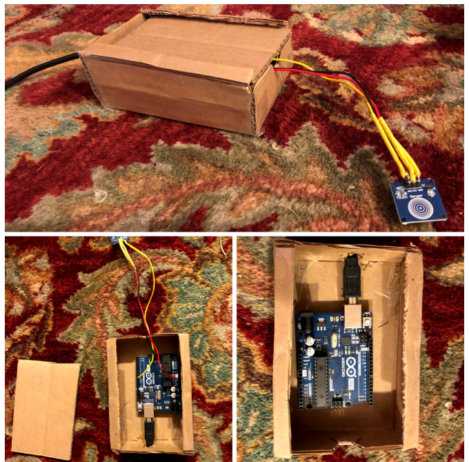
Figure 8. EMMA V2. Following this next round of iterations, I prototyped how the hardware components may be contained in a box.
