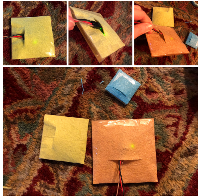
Figure 11. Templates covered in felt. The slit in the felt allows for easy access and removal of the touch sensor while simultaneously extending the sensor's range of contact.
